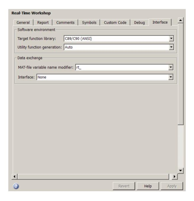
The Real-Time Workshop Interface pane includes the following parameters when the Real-Time Workshop product is installed on your system and you select an ERT-based target. ERT-based target parameters require a Real-Time Workshop Embedded Coder license when generating code.
