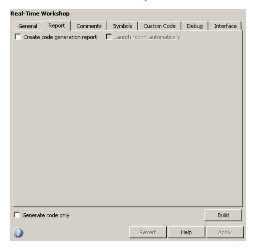
The Real-Time Workshop Report pane includes the following parameters when the Real-Time Workshop product is installed on your system and
