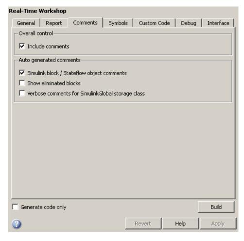
The Real-Time Workshop Comments pane includes the following parameters when the Real-Time Workshop product is installed on your system and
