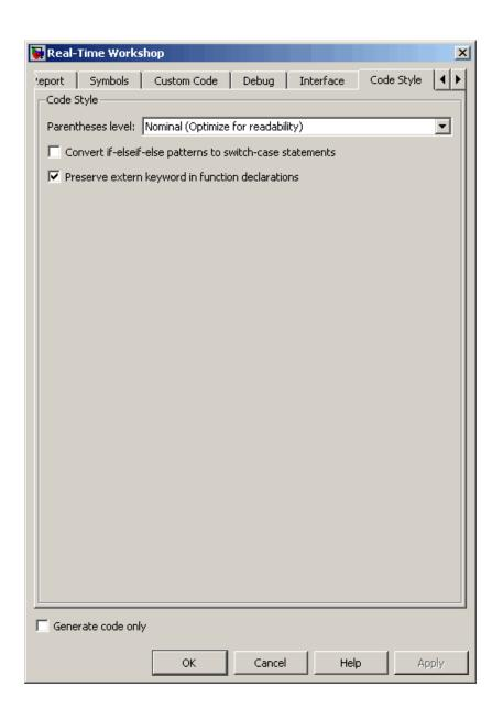
The following table describes the code style parameters for the Embedded MATLAB Coder **Real-Time Workshop** dialog box:
